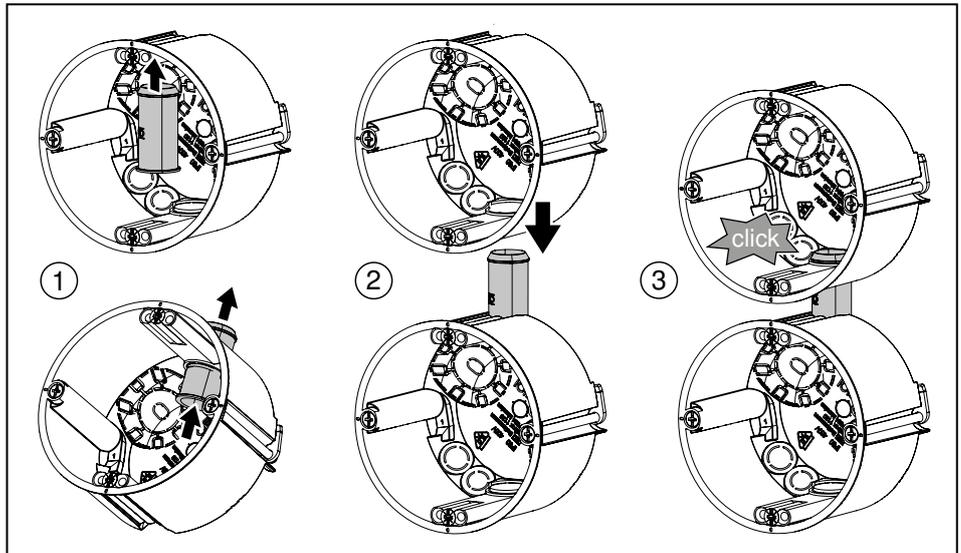
Fig. 13: Inserting and connecting connectors
