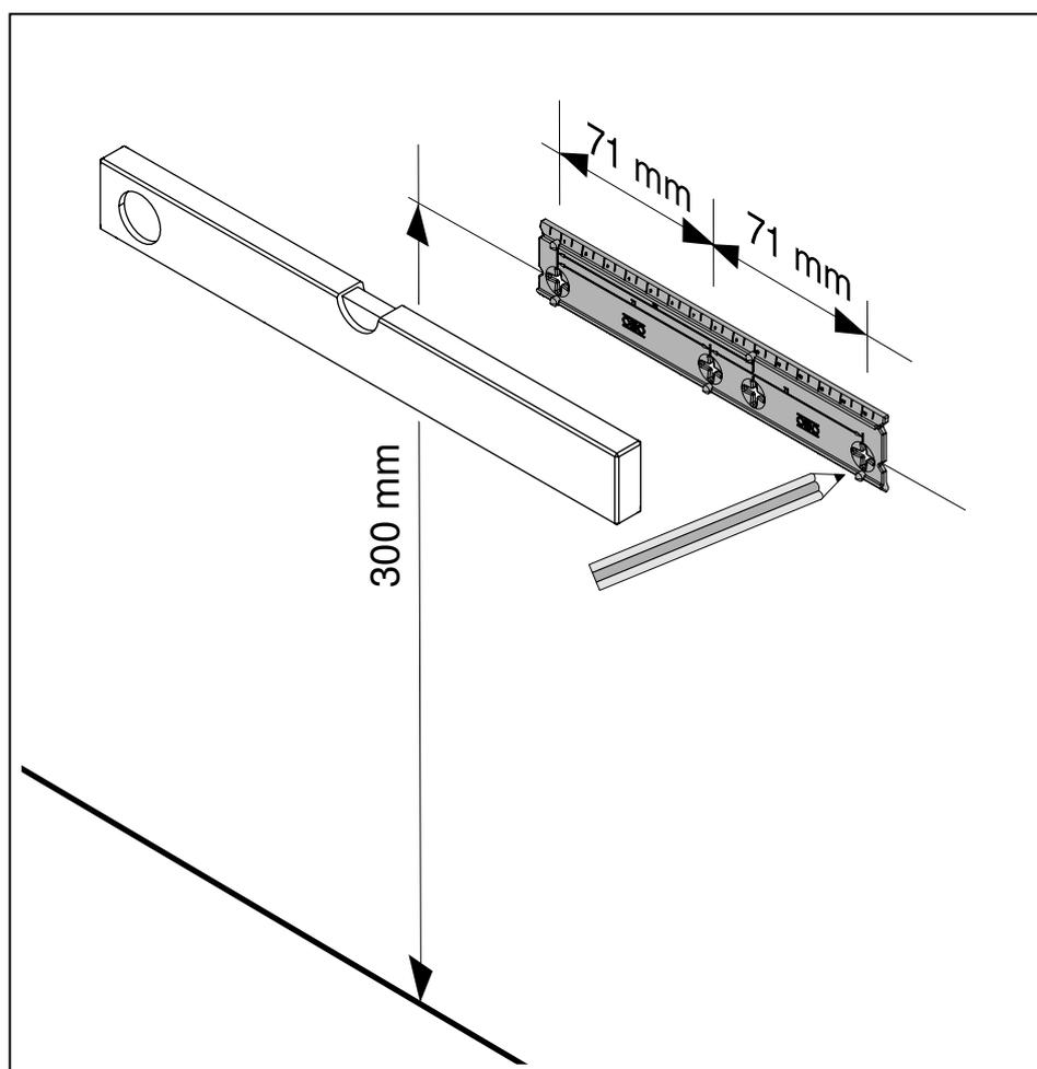
Fig. 5: Drawing on the drill hole
