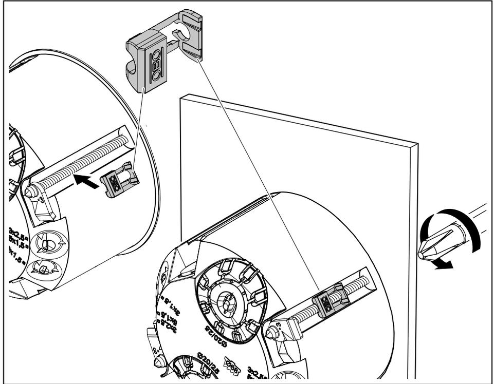
**Fig. 16:** Applying the fastening element
