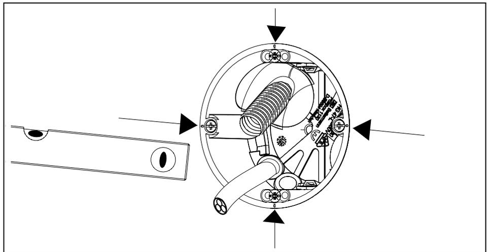
**Fig. 10:** Aligning the cavity wall box
