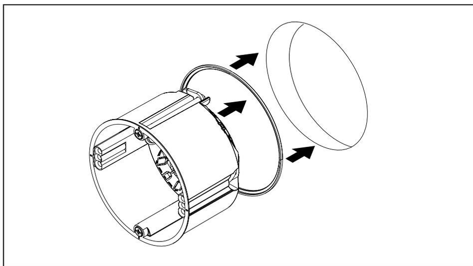
**Fig. 24:** Inserting the compensation ring
