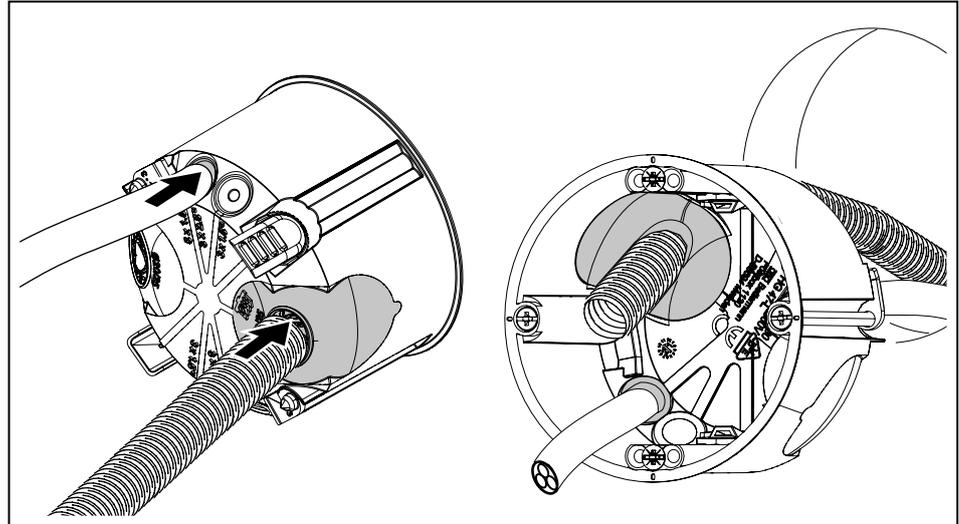
**Fig. 9:** Inserting the cable and corrugated pipe into the airtight cavity wall box
