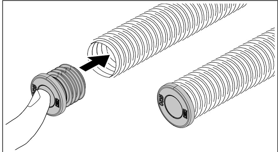
Fig. 25: Inserting the sealing plug
