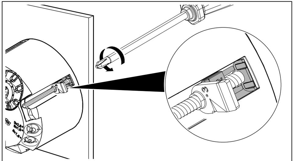
**Fig. 17:** Tightening the clamping lug
