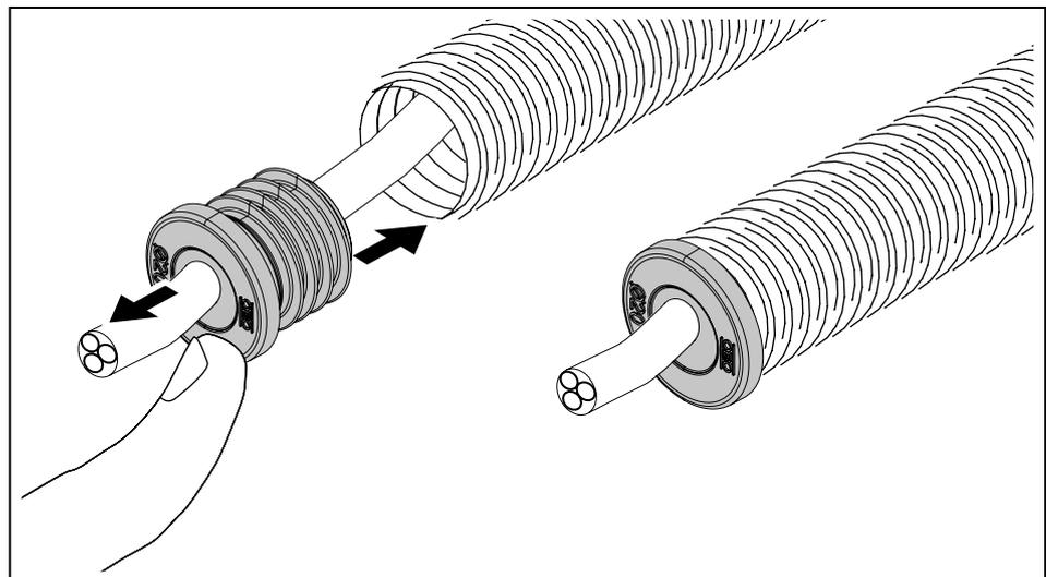
Fig. 26: Inserting sealing plug with cable
