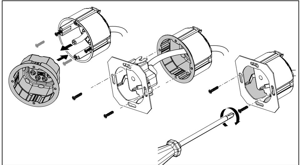
**Fig. 22:** Inserting a sealing insert with a device
