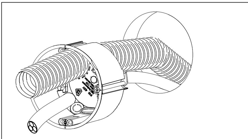
**Fig. 8:** Inserting the cable and corrugated pipe into the cavity wall box
