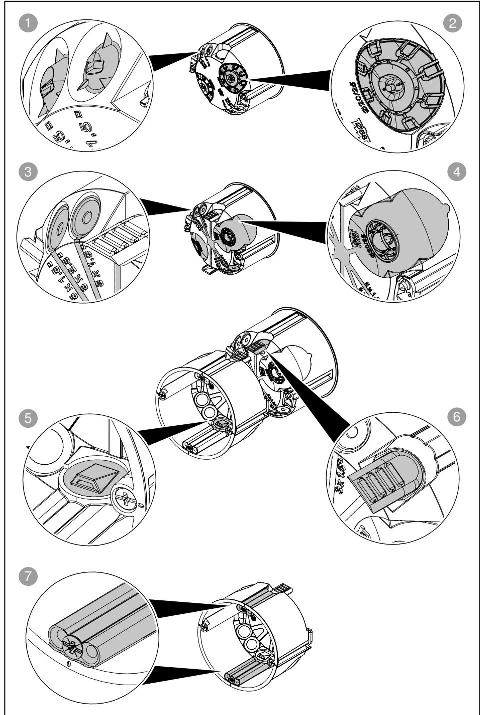
Fig. 3: Details, cavity wall boxes
