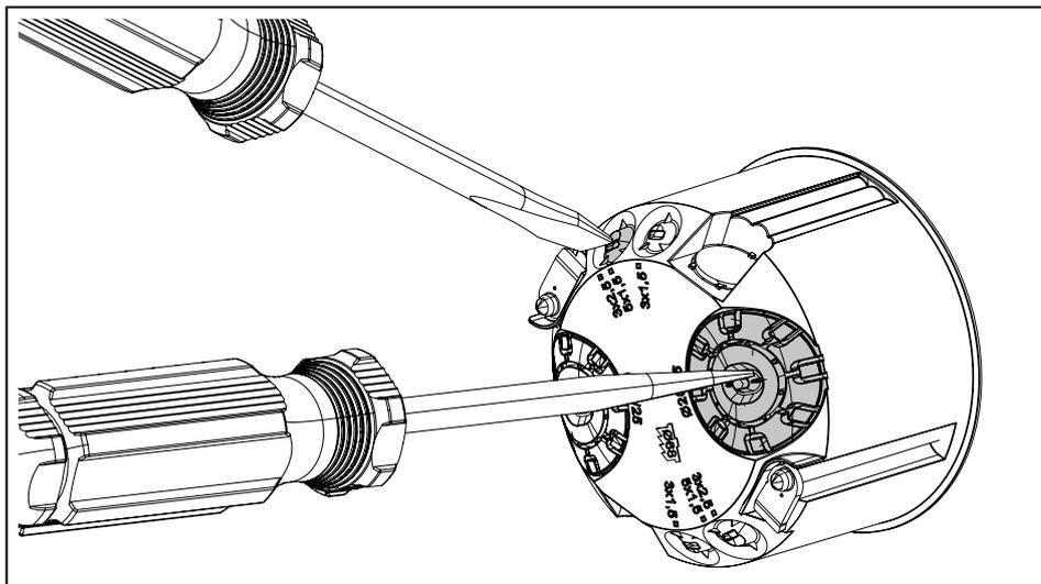
**Fig. 7:** Breaking out the break-out openings
