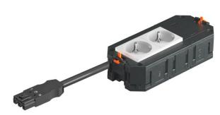
The ready-for-connection UTC3 universal support has 2 pre-installed 33° protective contact sockets in white of 16 A and one blanking cover for retroinstallation of an installation device of the Modul 45 or Modul 45connect series. Suitable for VL connection cables and device installation units of nominal size 2, 4, R4, 6 and  $^{\rm P7}$
