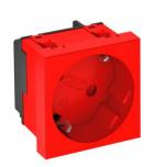
Protective contact socket, Single 33°, with increased touch protection, with screwless terminals, 2-pin, 16 A, 250 V $\sim$ , with connection terminals to IEC 60884-1
