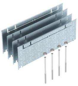
Height compensation set for underfloor boxes UZD350-3 with a construction height of 165 to 220 mm, consisting of four fall plates, four height adjustment screws and four rotary locks.
